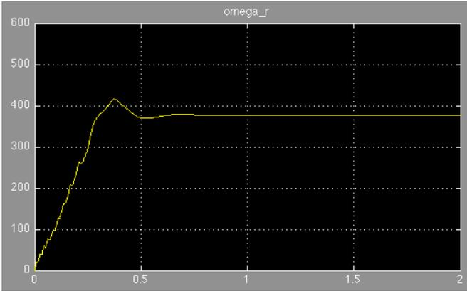
Fig. 4. Salient pole rotor speed [rad/sec] during start-up time [sec].
