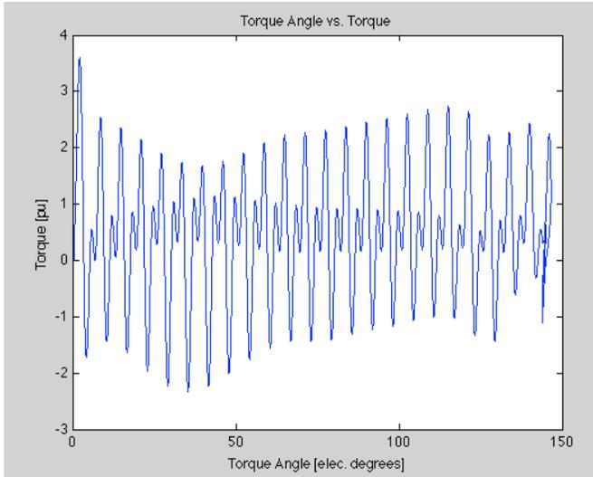
Fig. 9. Nonsalient  $\delta$ -torque characteristic.
