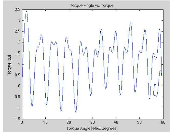
Fig. 11. Salient  $\delta$ -torque characteristic.
