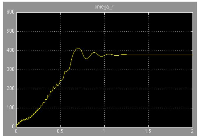
Fig. 3. Nonsalient pole rotor speed [rad/sec] during start-up time [sec].
