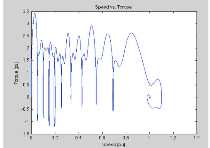
Fig. 2. Instantaneous torque dynamics of the salient pole LS-PMSM.
