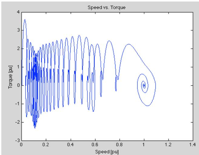
Fig. 1. Instantaneous torque dynamics of the nonsalient pole LS-PMSM.
