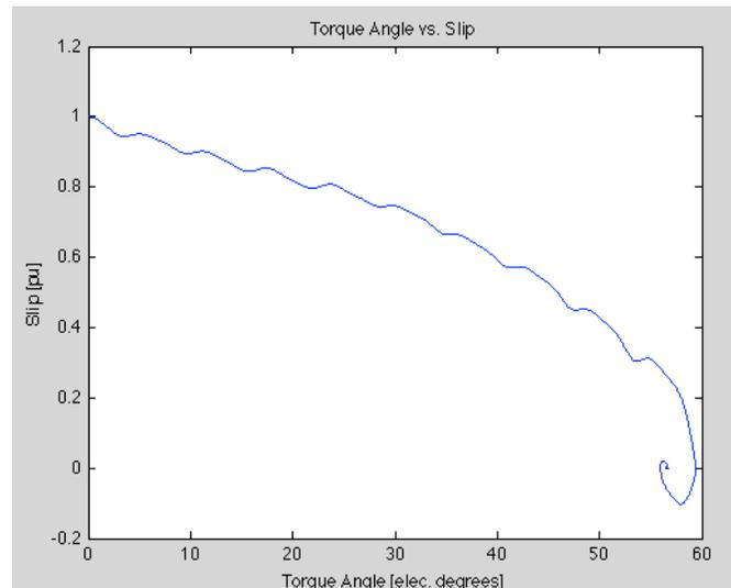
Fig. 7. Salient  $\delta$ -slip characteristic.
