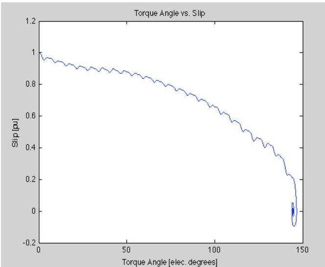
Fig. 5. Nonsalient  $\delta$ -slip characteristic.
